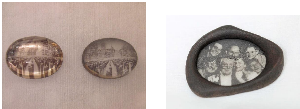
Left picture: The sample on the left (more bright) is made by silver on rock crystal and to the right (less bright) by aluminium on rock crystal. Right picture: Titanium oxide on silver, and after that enamel as passivation on top.
